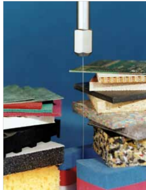
Various materials, cut with a pure waterjet.
